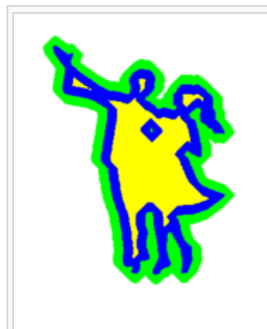
A shape (in blue) and its morphological dilation (in green) and erosion (in yellow) by a diamond-shape structuring element.
