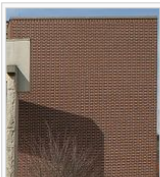
Fig.5: Subsampled image showing a Moiré pattern
