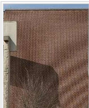
Fig.5: Subsampled image showing a Moiré pattern
